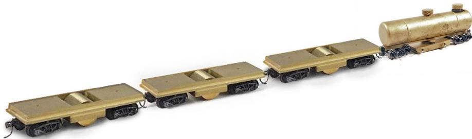
1. The La Mesa club uses this track cleaning car arrangement to daily clean their track (they run ~12 hours of trains every day). The lineup consists of one CMX Clean Machine car with mineral spirits solvent and three Centerline cars each with a dry wiper roller to remove the residue.
