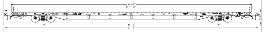
BUILT BY: EBENEZER RAILCAR SERVICES, INC DATE BUILT: 2020 PURCHASED FROM: ERS, INC PLACED IN SERVICE: 2020 36 INCH WHEELS: **BEARINGS:** 6½ X 9 COUPLERS: UNDERFRAME: CUSHIONED EOC - NEED GROUP DESIGNATION YOKES: NEEDTYPE DESIGNATION FLOATING AIRBRAKES: WABTECH ABDX-L AAR RULE 13, GROUP U SIDE MOUNT HANDBRAKE: LIGHTWEIGHT - LBS.: 81,500 CAPACITY - LBS.: 204,500
