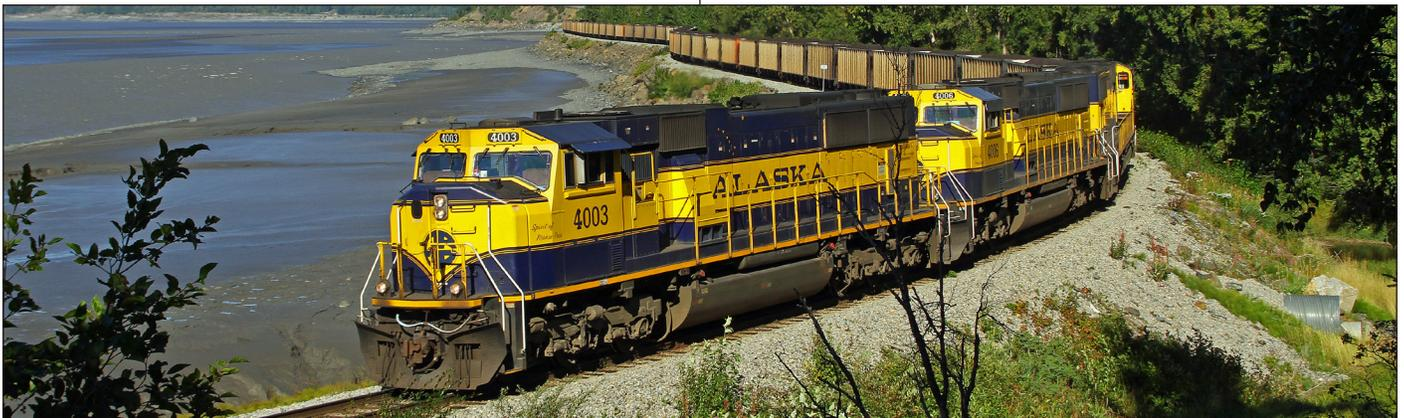
**SD70MAC locomotives haul coal-filled hoppers from the Healy coal mine to the loading facility in Seward. (photo by Frank Keller)**
