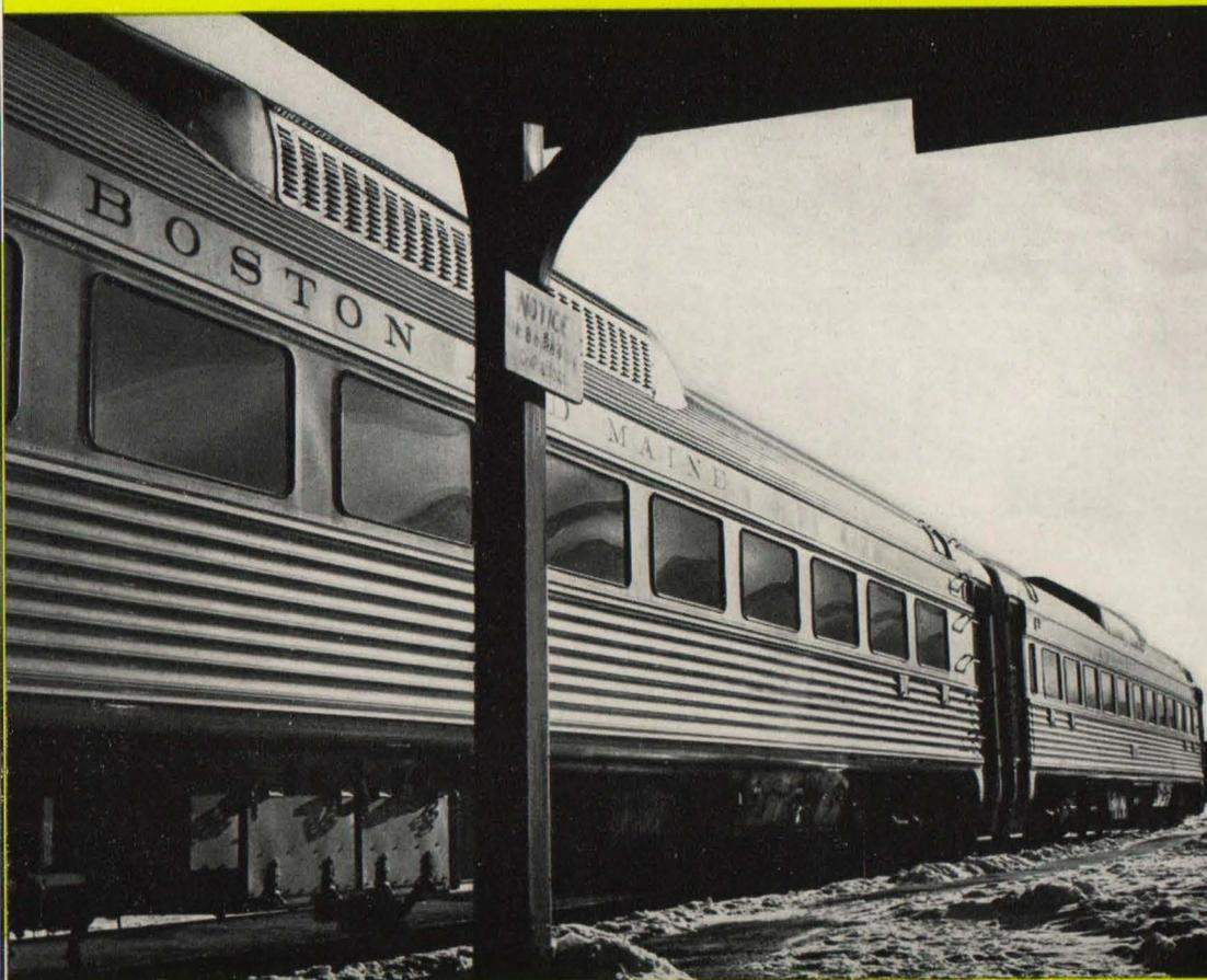
RDCs may be operated in any multiples the traffic requires, with all cars controlled from a single station.
