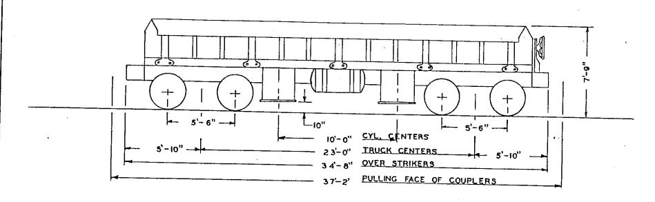
BUILT BY AUSTIN WESTERN CO. DATE BUILT 1941 REBUILT BY PURCHASED FROM KENNECOTT COPPER CORP PLACED IN SERVICE 1964 WHEELS TRUCKS **AXLES** 5 XIO" FRICTION **BEARINGS** UNDERFRAME STEEL LIGHTWEIGHT-LBS. 65,000 CAPACITY 100,000 LBS. 30 YDS. **COUPLERS** E-60 Y-40 YOKES **AIRBRAKES** K2 10'X12" HANDBRAKE **POWER**
