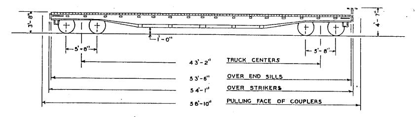
GUNDERSON BROS. ENGINEERING CORP. BUILT BY DATE BUILT 1964 REBUILT BY PURCHASED FROM GUNDERSON BROS ENG'G CORP. PLACED IN SERVICE 1964 WHEELS 33 **TRUCKS** BARBER **AXLES** 6"X 11 **BEARINGS** TIMKEN 6"XII" **UNDERFRAME** STEEL LIGHTWEIGHT -LBS. 54,100 CAPACITY -LBS. 140,000 **COUPLERS** TYPE BE-60A-HT YOKES Y - 40**AIRBRAKES** AB 10"X12" HANDBRAKE DROP SHAFT
