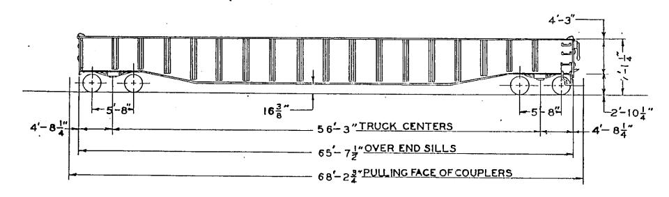
BUILT BY PRESSED STEEL CAR CO. 3 - 44 DATE BUILT REBUILT BY PURCHASED FROM SURPLUS PLACED IN SERVICE 4-5-47 WHEELS TRUCKS UNIT BARBER STABILIZED AXLES 6'X II" BEARINGS FRICTION UNDERFRAME STEEL LIGHTWEIGHT- LBS. 59,500 CAPACITY 140,000 CU.FT. 1,777 E-60+N.M.& S.C.CO COUPLERS VERTICAL W/ HORIZ. PIN AB - 10"X 12" CYL. YOKES **AIRBRAKES** HANDBRAKE
