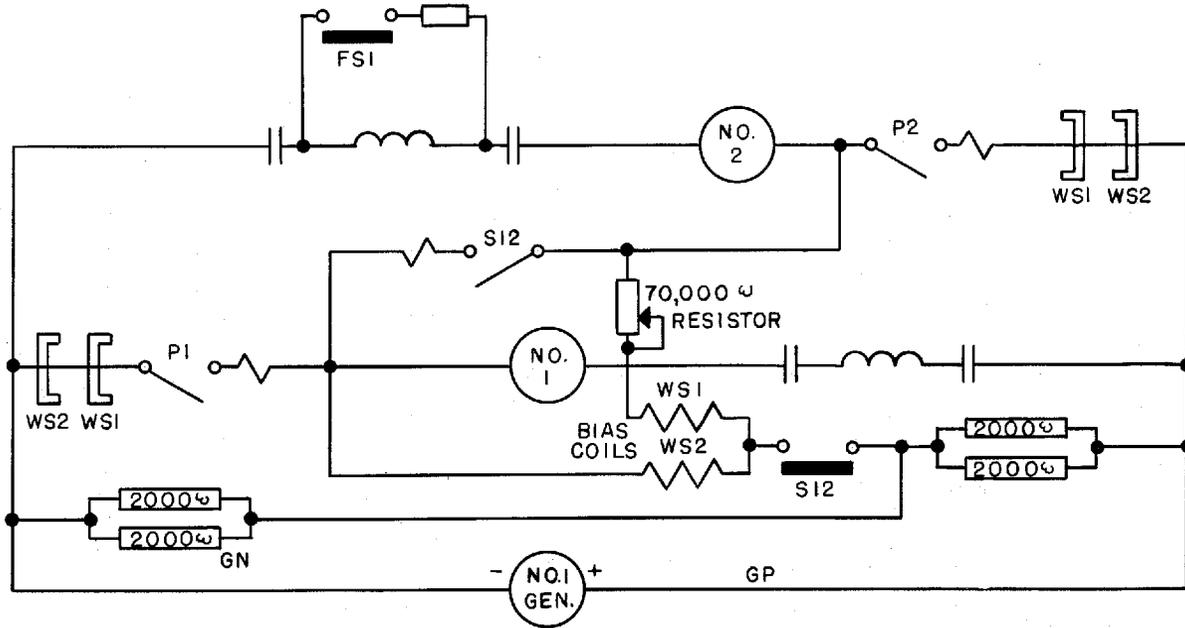
High Speed Wheel Slip Circuit
