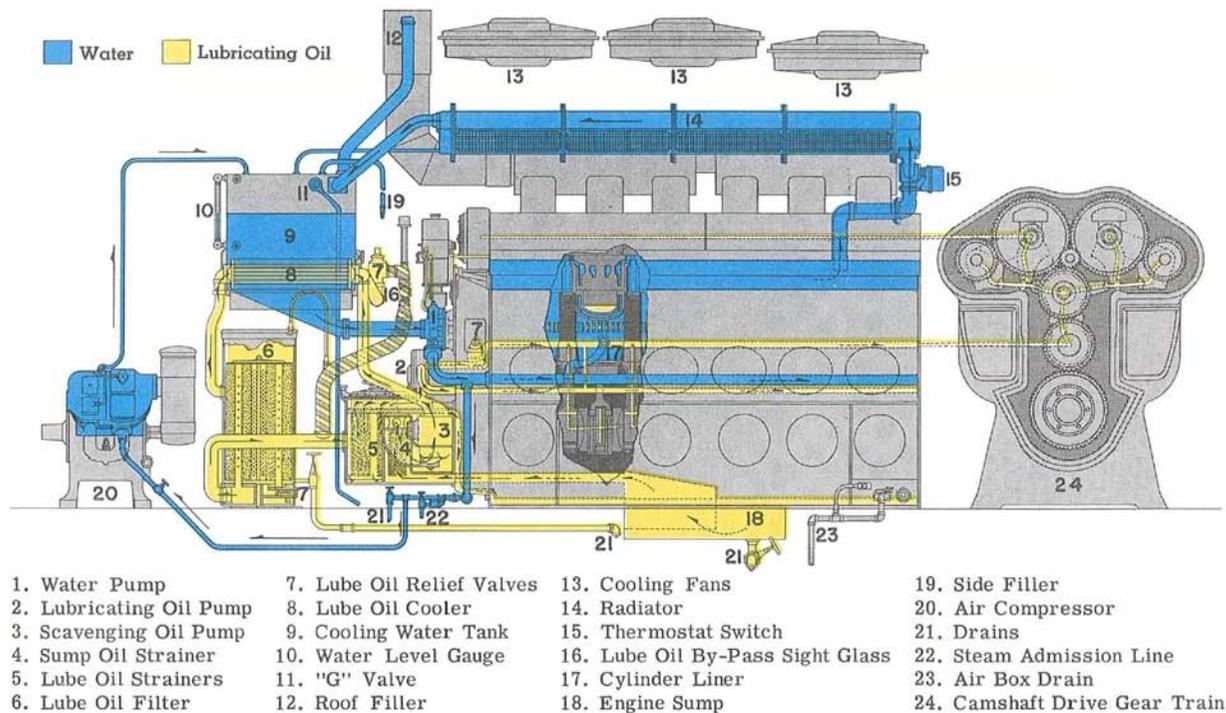
Fig. 4-1 - Schematic Of Cooling And Lube Oil Systems
