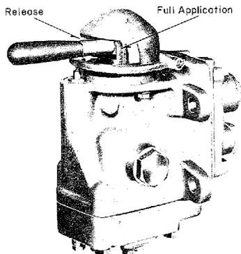
position. The brake valve is of the self-lapping type, and maintains the brake cylinder pressure as set by the handle position. Quick release of the locomotive brakes following automatic application is obtained by depressing the independent brake valve handle in the full release position.
