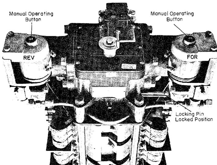
Reverser Switch - Locked In Neutral
