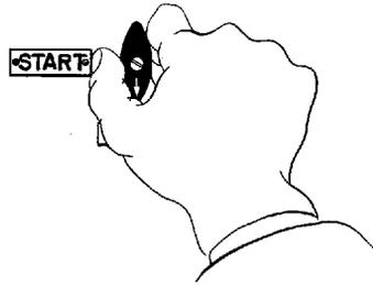
Placing Engine On the Line
